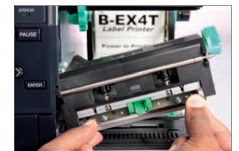
Snap-in printhead reduces maintenance downtime to a minimum
